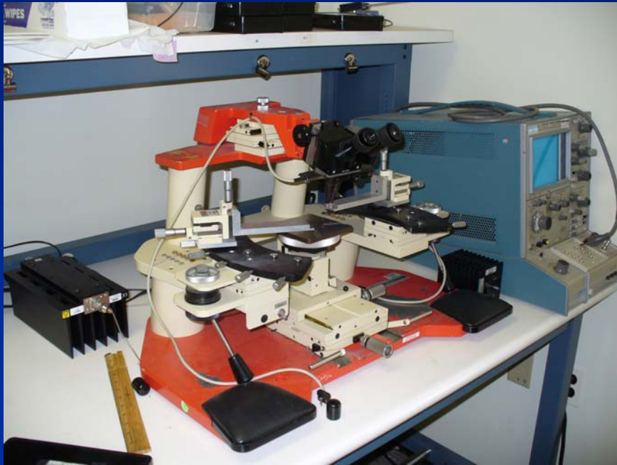
On-Wafer Probe Station
