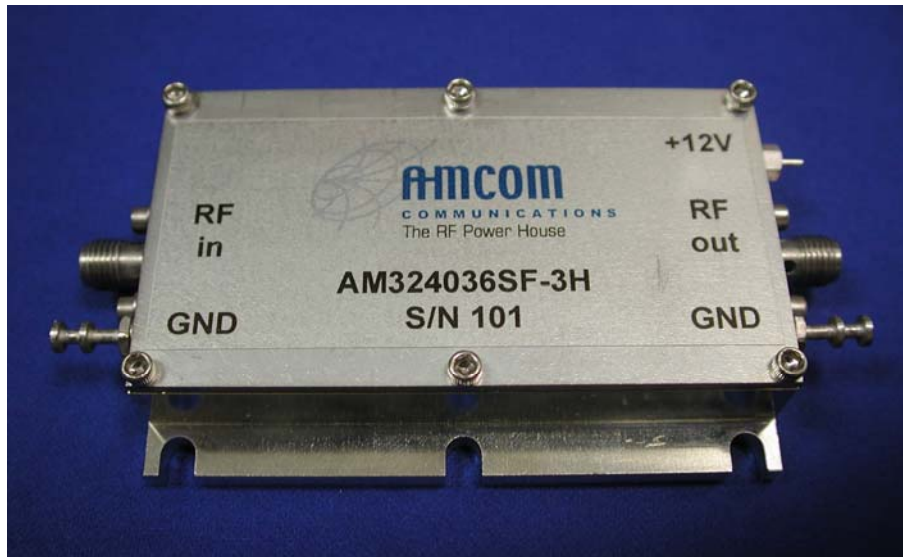
Figure 6: Photograph of PA Module
