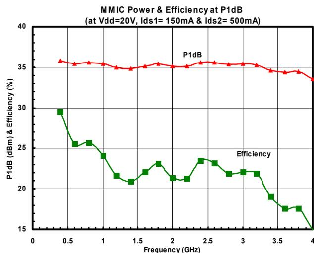
Fig. 1: Output power  $P_{1\text{dB}}$  and efficiency as a function of frequency.  $P_{1\text{dB}}$  is very flat, from  $35\text{dBm} \pm 0.5\text{dBm}$  from 20MHz to 3500MHz.
