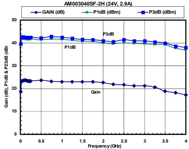
Fig. 6. Output power P1dB and P3dB versus frequency
