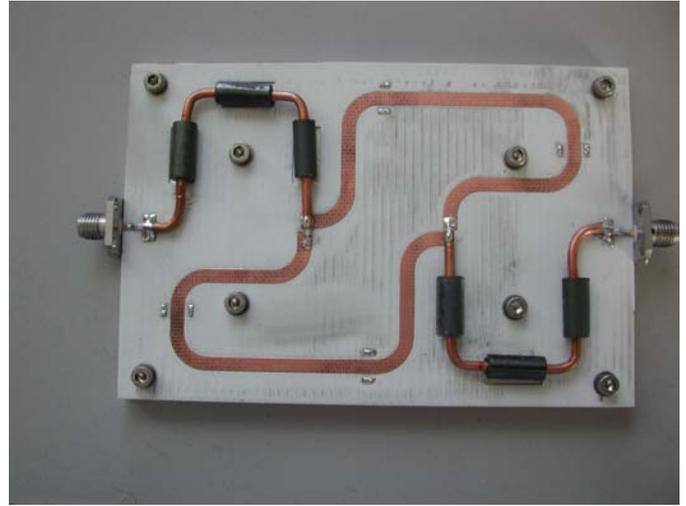
Fig. 3a. Photograph of a prototype 2-way balun.
