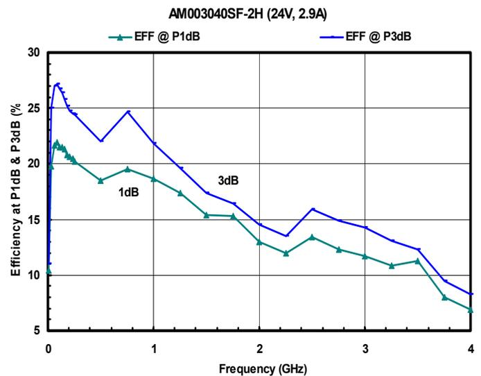
Fig. 7. Efficiency at P1dB and P3dB versus frequency
