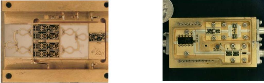
Figure 4: Examples of Carrier Mounted MMICs
