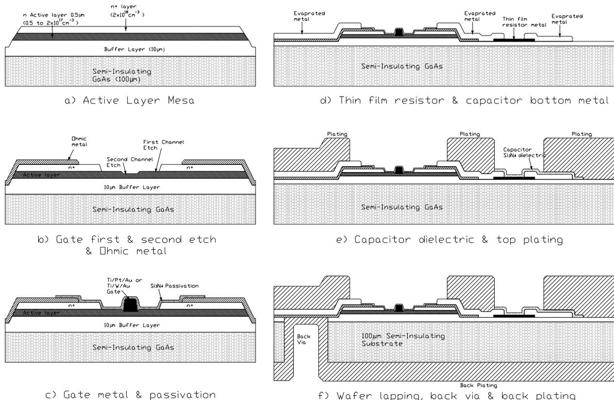
Figure 3: Typical Fabrication Steps for a GaAs MESFET Process
