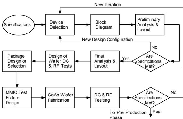
Figure 6: Block Diagram of MMIC development phase
