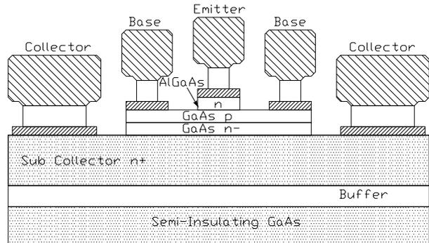
Fig. 2: Typical HBT Structure
