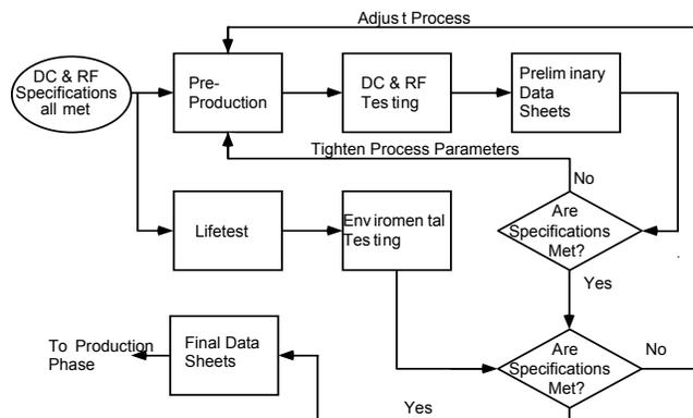
Figure 7: Block Diagram of MMIC production phase
