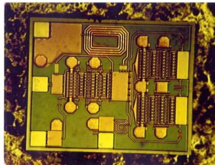
Figure 11: 3Watt Broadband MMIC using HiFET
