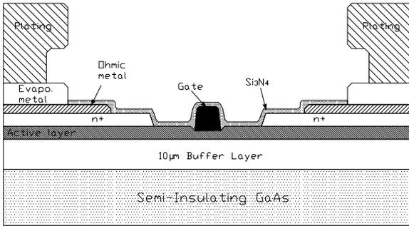
Fig. 1: Typical pHEMT Structure
